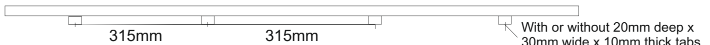
LB IR 330 - 330mm tall by 1260mm long - Approx 20mm thick - Single sided detail
